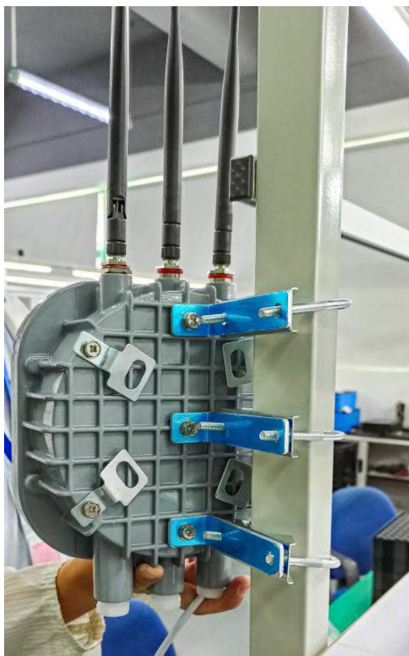
Figure3.1-R Insert the U-bolts to the L-shape steel
